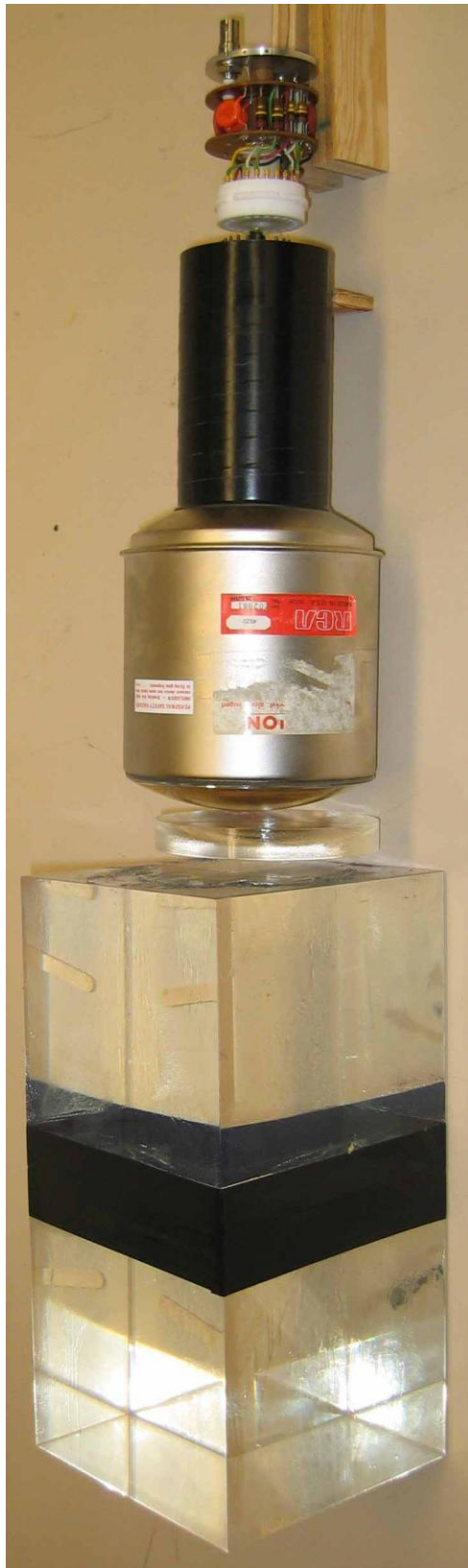
The components of the muon detection experiment before final assembly.
