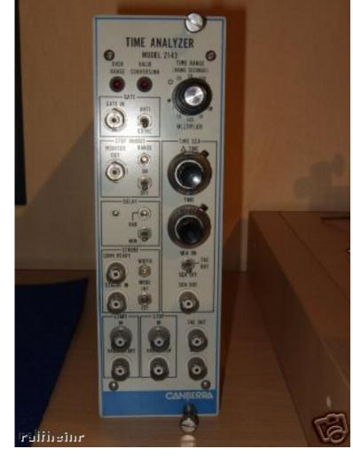
CONVersion READY –Output pulse specification identical to VALID START. Active from end of DELAY period. Duration set by CONV READY WIDTH control. Range set by internal jumper, 1 to 20  $\mu$ s or 10 to 200  $\mu$ s; shipped in 1-20  $\mu$ s position. Indicates period when STROBE input will initiate output pulse.
