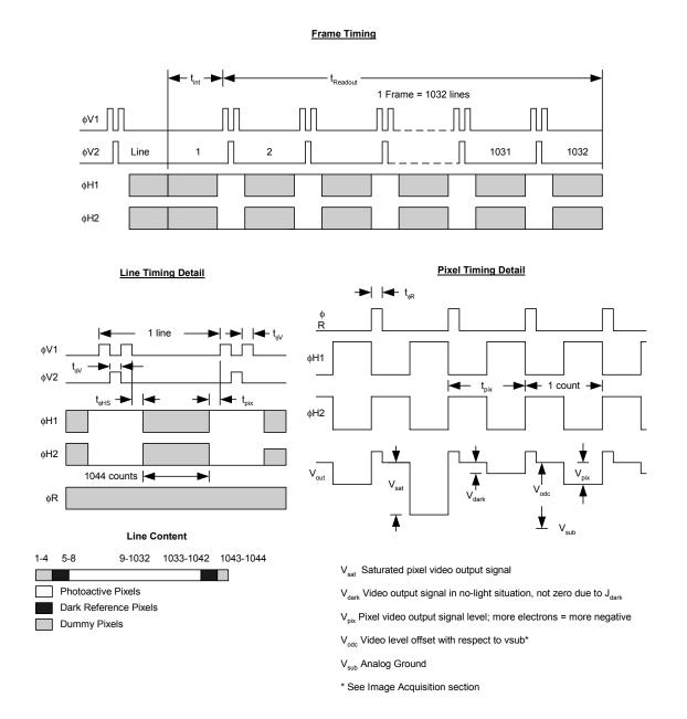
Figure 4 - Timing Diagram
