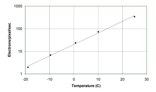
Figure 6 - Dark Current as a Function of Temperature
